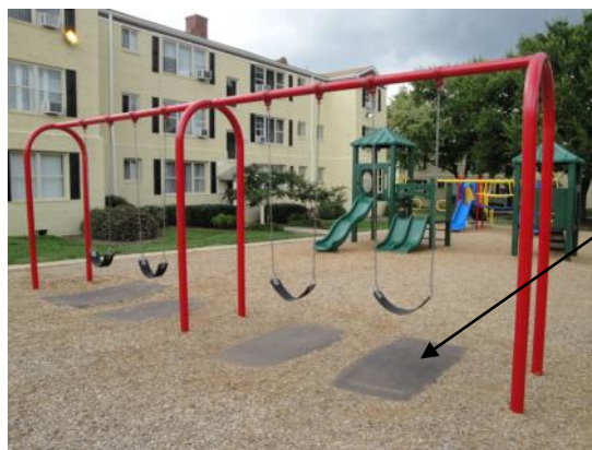
Example of Woodcarpet pvc wear mats installed below swings keeping this area accessible.
