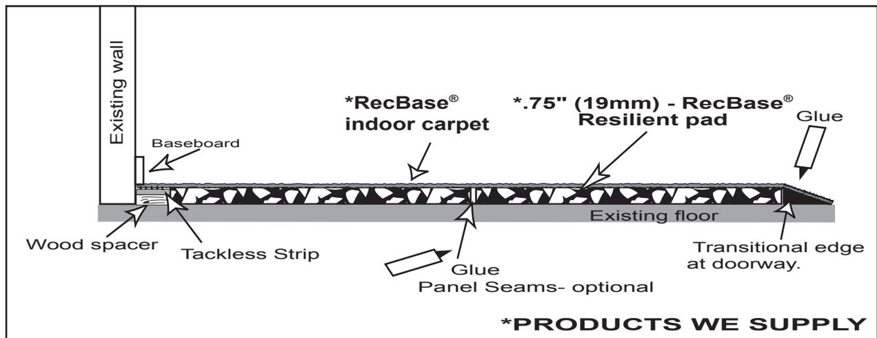
**E. Application:** Indoor play area installed over an existing hard surface such as concrete or wood floor.
